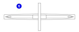
**Double spike** made of ABS and caps made of PE.
